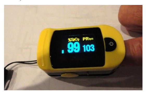
The pulse oximeter, or Pulse Ox, is an electronic device that measures the saturation of oxygen carried in your red blood cells. The device uses a cold light source that shines a light through the fingertip, making the tip appear to be red. By analyzing the light from the light source that passes through the finger, the device is able to determine the percentage of oxygen in the red blood cell.
