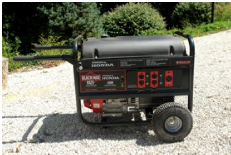
Figure 24. Portable Electrical Generator, BlackMax, Model PM0496500, 13 HP, 6500 running watts, 8125 max watts
