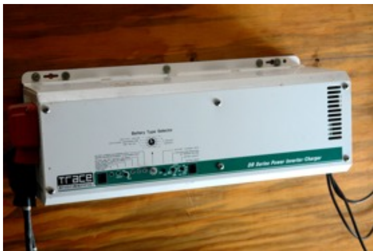
Figure 28. Trace Power Converter/Charger
