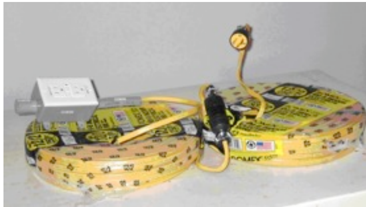
Figure 26. Two Extension Cords 120 Volt, 250 Feet Each
