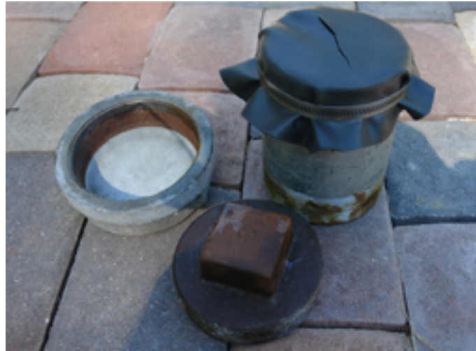
Metal Cap, Plug & Restrictive Flow Vent Pipe
