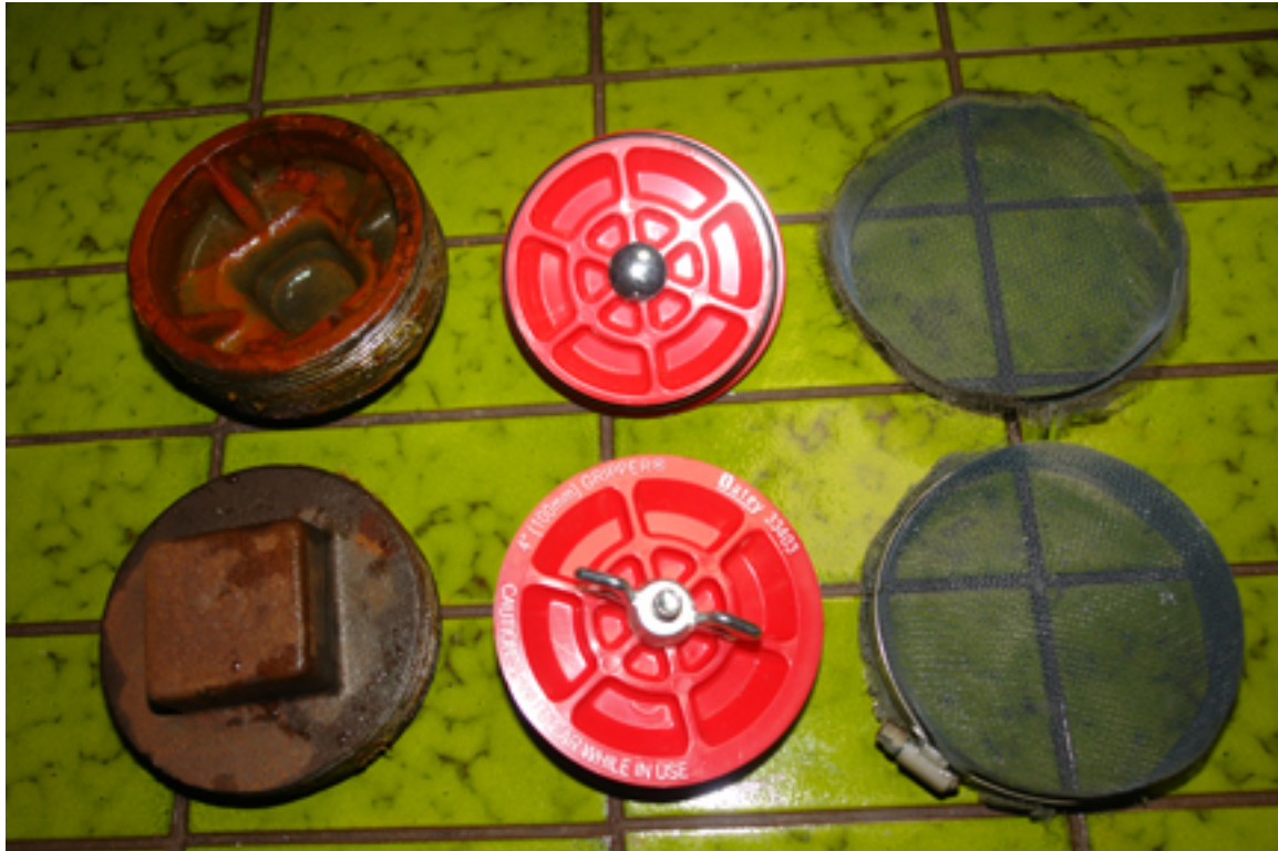
Square Head Threaded Metal Plugs, Oatey Gripper Test Plugs, Aluminum Screen Exterior Coverings
