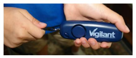
Another bit of technology that has appeared recently is small personal alarms. This is a photograph of a personal alarm by Vigilant. It easily fits in a shirt or pants pocket. It has a ripcord activation system that prevents false alarms. Pull the wrist strap with attached grenade style
